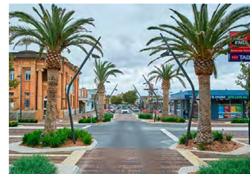
Raised pedestrian threshold with greening gateway
